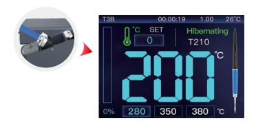
Handle being placed in the holder for a long time, the temperature will automatically drop to the preset sleep temperature.
